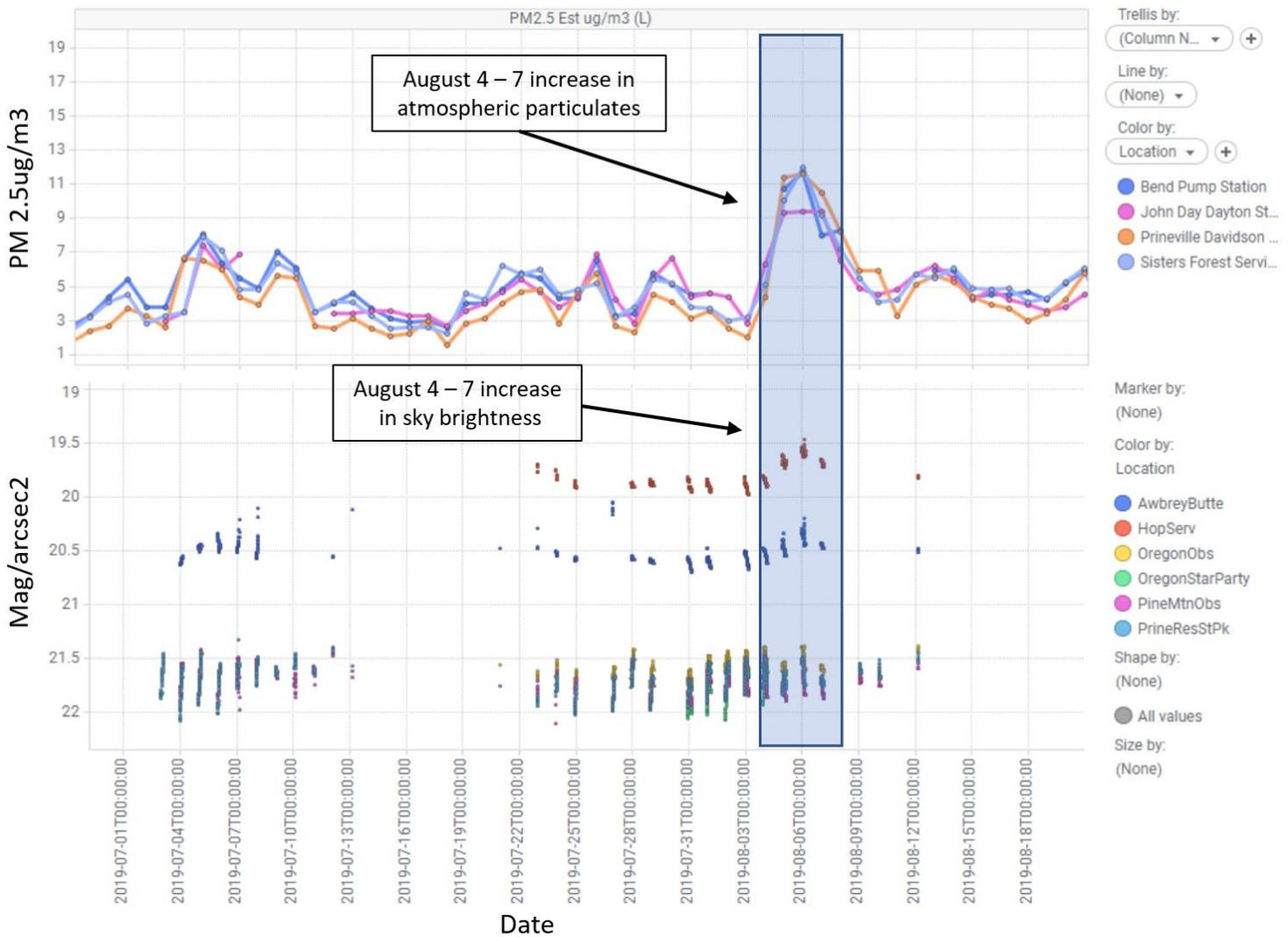
The SQM data have been calibrated to each other by analyzing a two-week data set during which all the SQMs were mounted together at the Awbrey Butte site. Data from each SQM was adjusted up or down to reach the mean value recorded by all of the SQMs together. The adjustment was from 0.00 to 0.03 mag/arcsec2.
