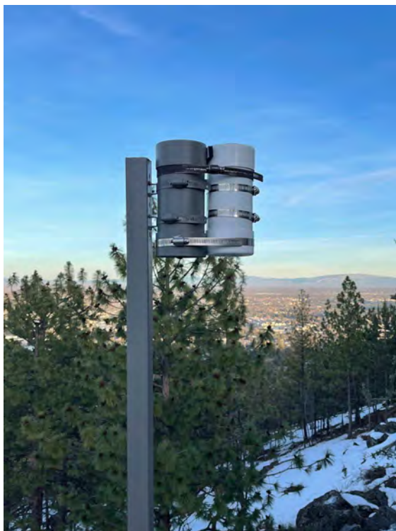
Figure D1. New and old SQMs running in parallel at two different sites, with the goal of assessing aging phenomena of the SQM unit. Awbrey Butte site on the left, Prineville Reservoir State Park on the right.
