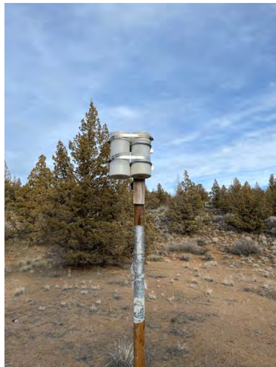
Figure D1. New and old SQMs running in parallel at two different sites, with the goal of assessing aging phenomena of the SQM unit. Awbrey Butte site on the left, Prineville Reservoir State Park on the right.
